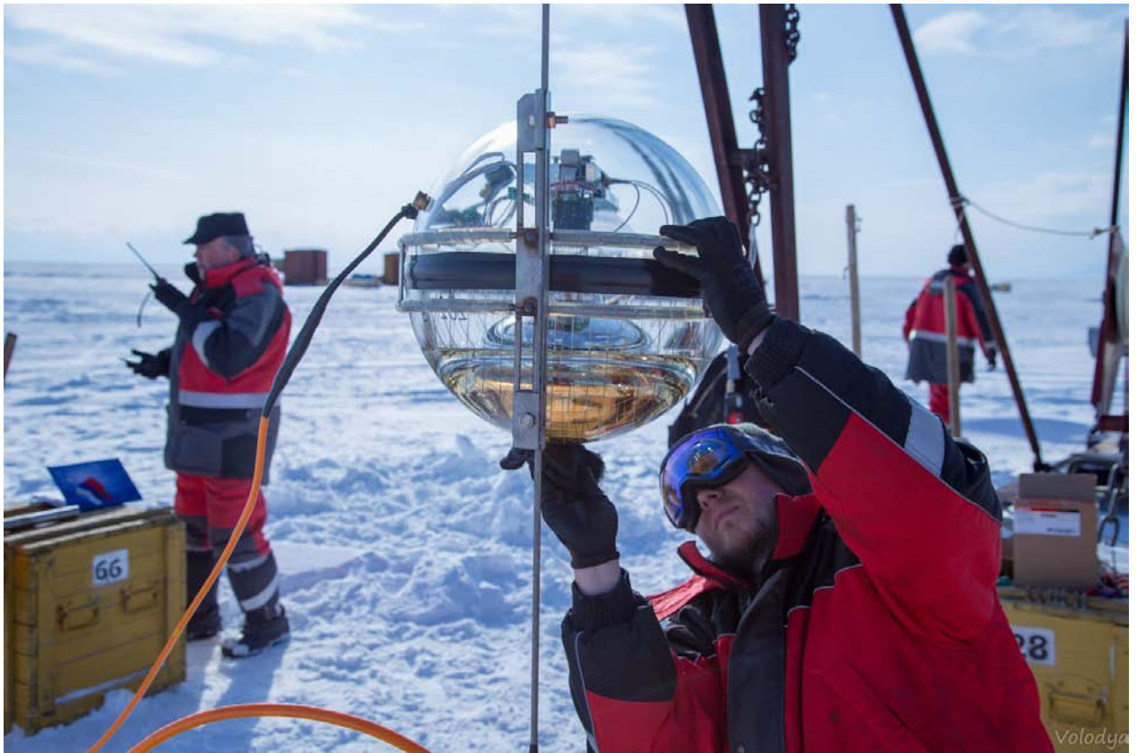
Figure 2. Participants of the Baikal experiment prepare a Cherenkov radiation detector, also known as an optical module, for deploying under the ice on Lake Baikal. The photomultiplier tube and other electronics are placed inside a transparent ball that can withstand the pressure of one and a half kilometers of water. This is a part of the telescope that collects information about faint flashes that accompany the interactions of neutrinos in water and sends it through a cable to the shore. Photo by Bair Shaybonov.
